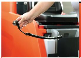
The on-board charger enables charging of the battery at any conventional 220/230V mains outlet.
